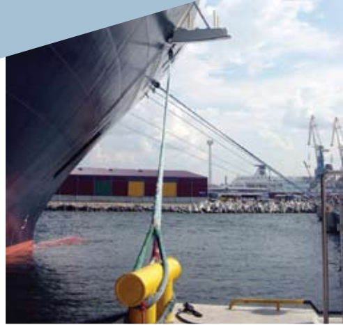
The forespring stops the ship moving forward. Head lines in the distance.
