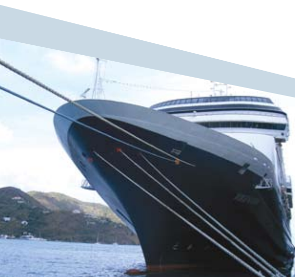
The Volendam tied up alongside. Note the five lines - two head lines and three breast lines configuration.
